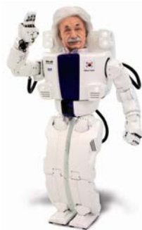
The Albert Hubo android has 66 degrees of freedom and is driven by maxon motors.
